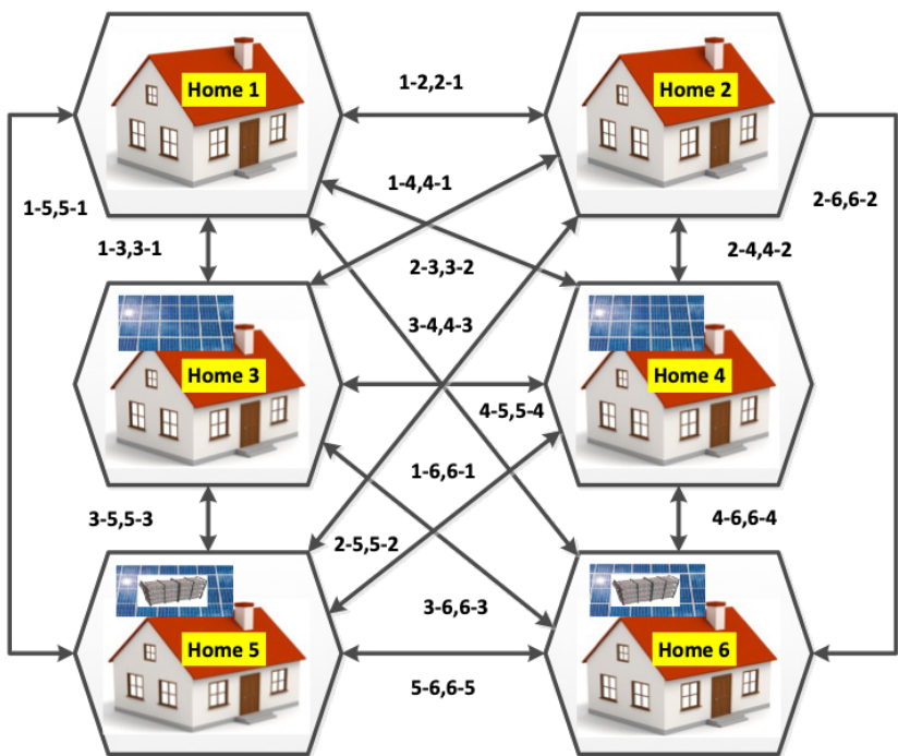
Figure 5. Decentralized Cooperative Community Microgrid Design.
