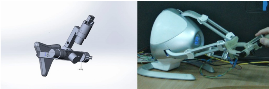
Figure 10. Custom designed grip to provide extra 3-degree of freedom.
