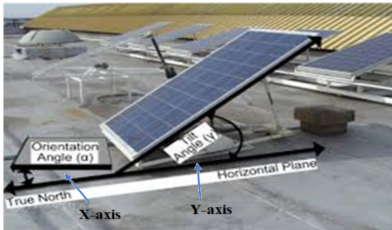
Figure 1. The tilt and orientation angles of a PV module. Source: (Asowata, Swart, & Pienaar, 2012).
