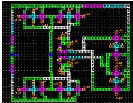
Figure 13. QCA Implementation of D Flip Flop used in Proposed Circuit.
