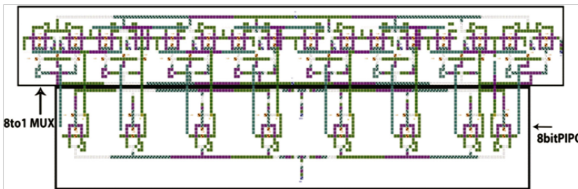
Figure 11. Proposed Circuit (Universal Shift) PIPO-8-Bit.
