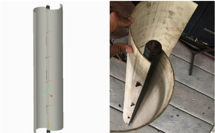
Figure 1. AutoCAD vs Hardware of Blades and Shaft.
