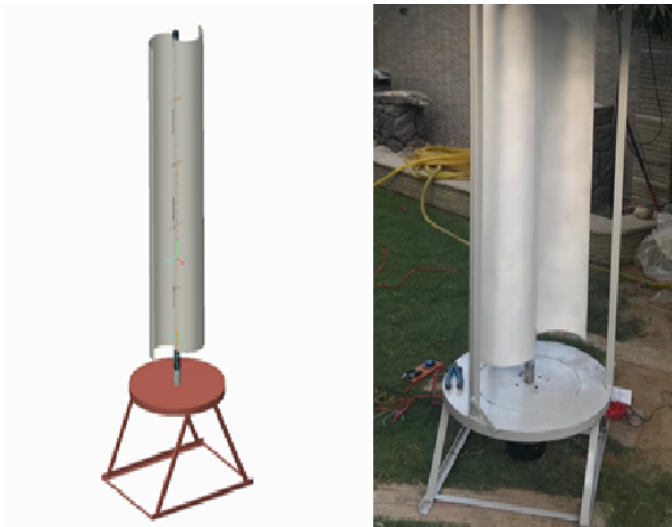
Figure 6. AutoCAD vs Hardware of S-rotor.
